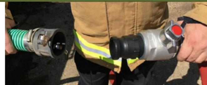
The new coupling fits directly to most bulk water supplies
